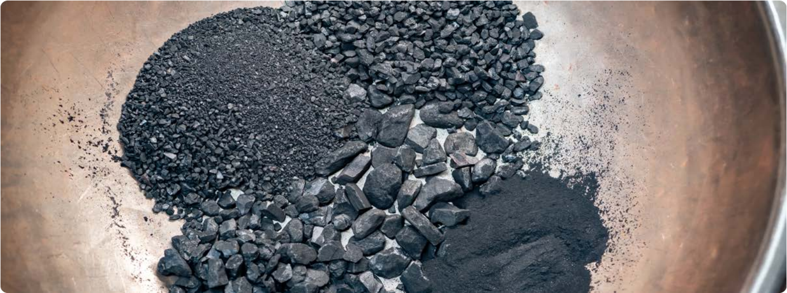
Lump ore - post reduction (in the furnace) tumbled and sieved to different sizes.
