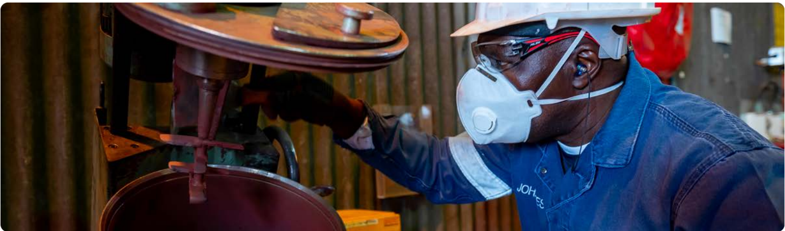
Johannes Kgaxise, Lab Technician, preparing the roller to make briquettes.
