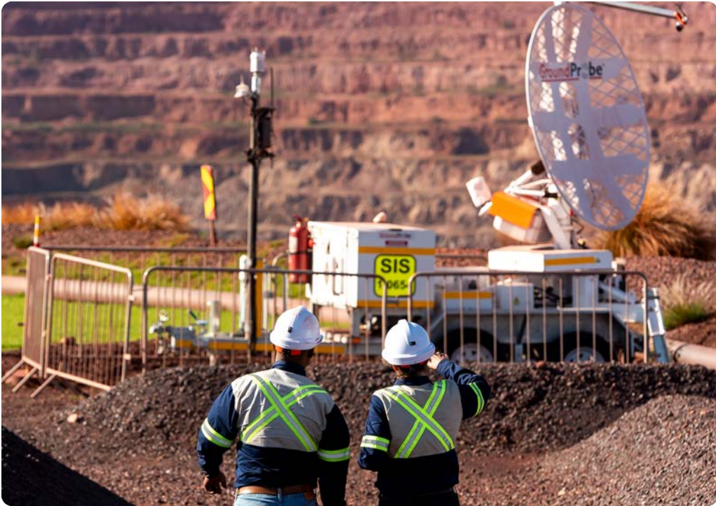
GroundProbe radars installed at both Sishen and Kolomela to continuously monitor slope stability and associated emergency evacuations triggers.
