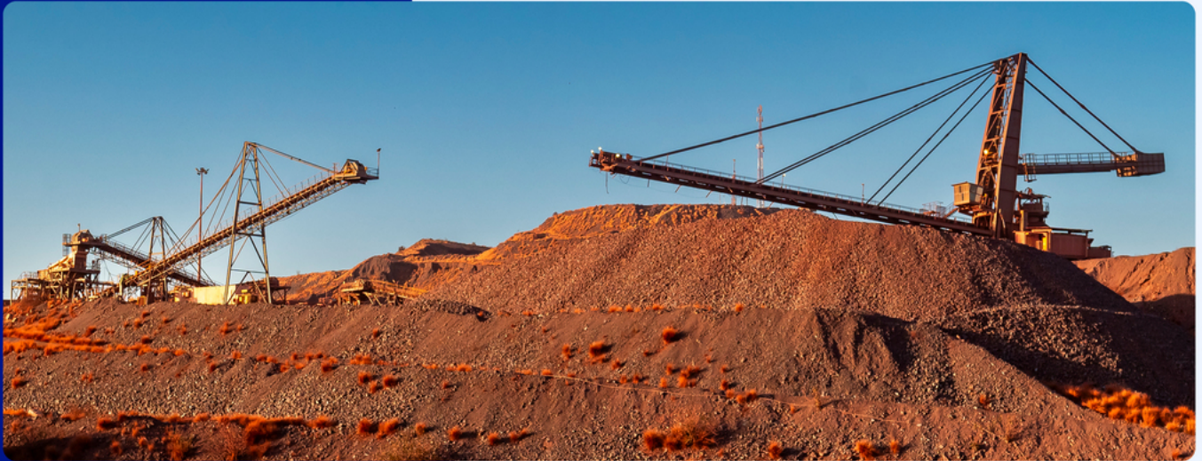
The link conveyor system at Sishen mine provides ore feed flexibility from the Jig crusher circuit to the DMS plant.
