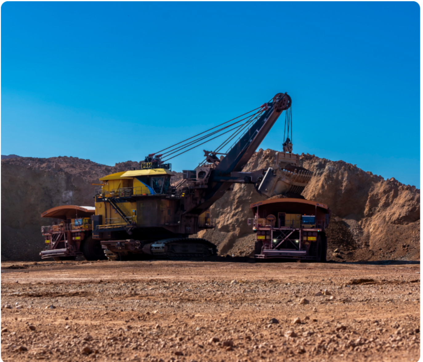
Double-sided loading of waste material at Sishen mine; using a P&H 4100 XPC Rope Shovel matched with Komatsu 960E haul trucks.
