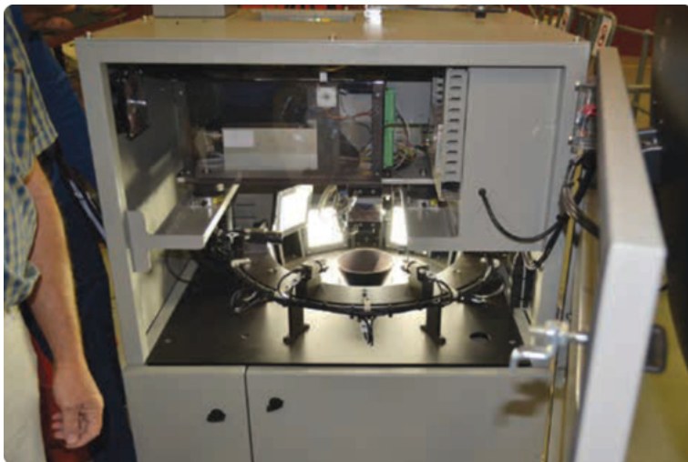
RhoVol (developed by De Beers Technologies SA): Following mass measurement, each particle is dropped into space where seven cameras capture silhouettes, which are processed to accurately determine volume and shape
