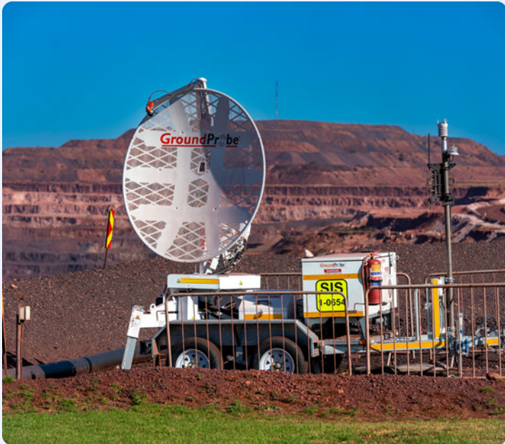
The GroundProbe berm monitoring system monitors any movement or height deficiencies in the berms and alerts the control room of any movements.
