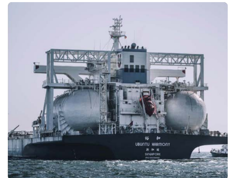
LNG dual-fuelled Capesize+ vessel, the Ubuntu Harmony, delivering an estimated 35% reduction in CO 2 emissions compared to ships fuelled by conventional marine oil fuel. T
