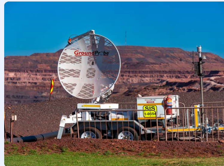
The GroundProbe berm monitoring system monitors any movement or height deficiencies in the berms and alerts the control room of any movements.
