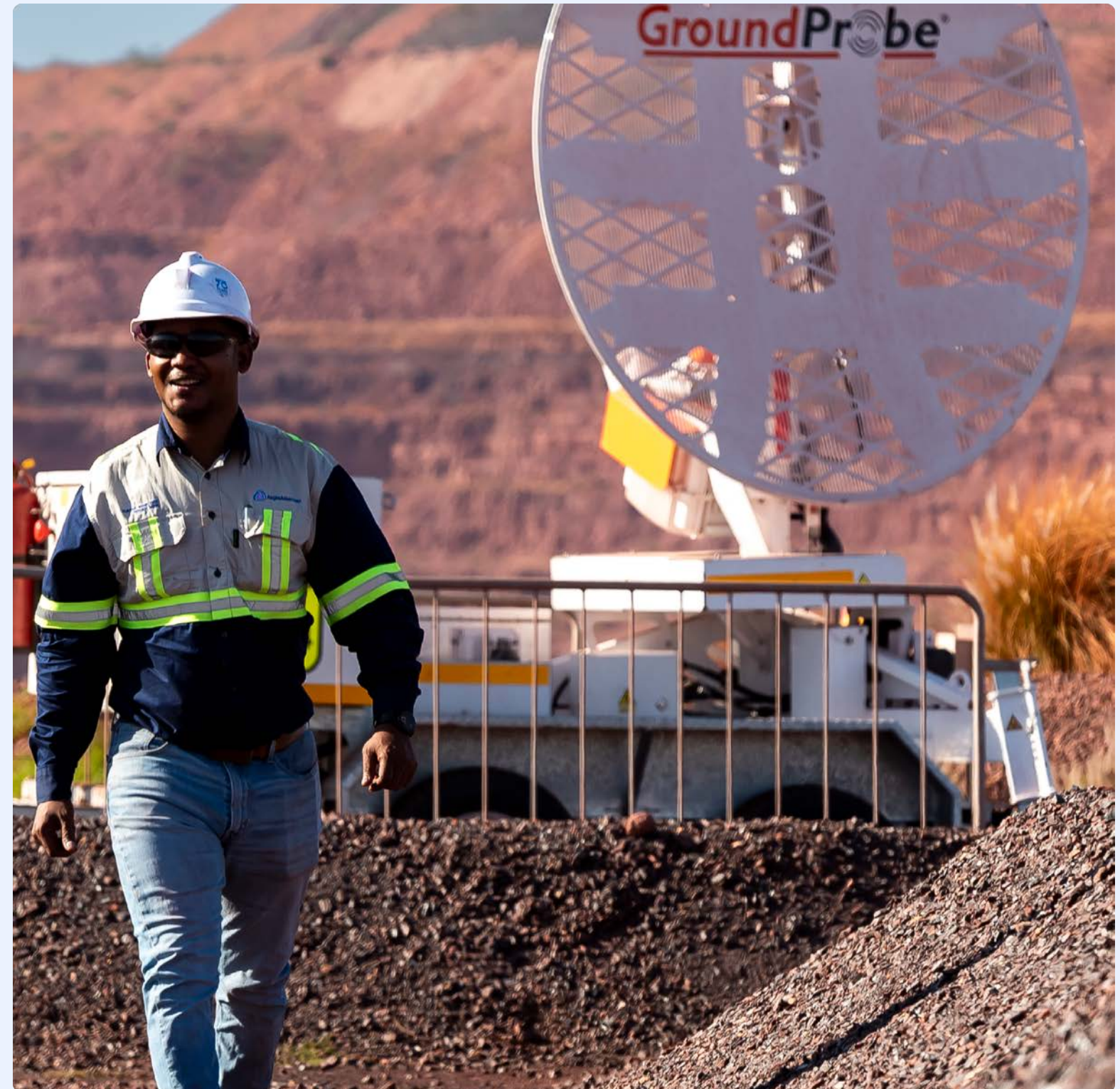
Ground stability radar is used in several locations in the various pits of the mines to monitor any movement in the pit walls.
