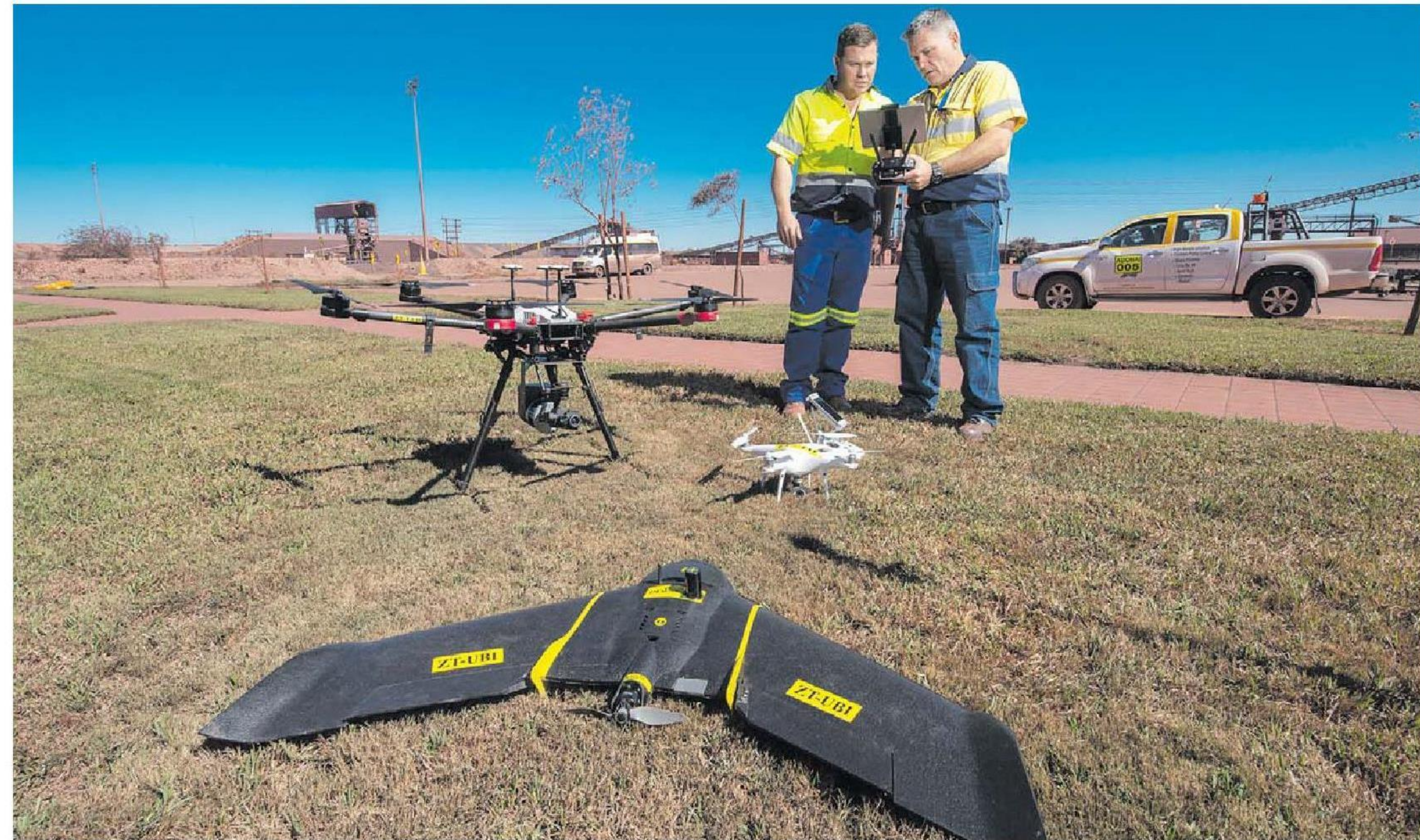
TECHNOLOGY. Kumba mines uses drones to reduce the need for employees to do physical blast clearances.
