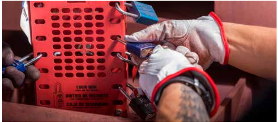
Image: Employees performing an isolation and lock-out procedure at the life-of-mine truck workshop at Sishen mine.
