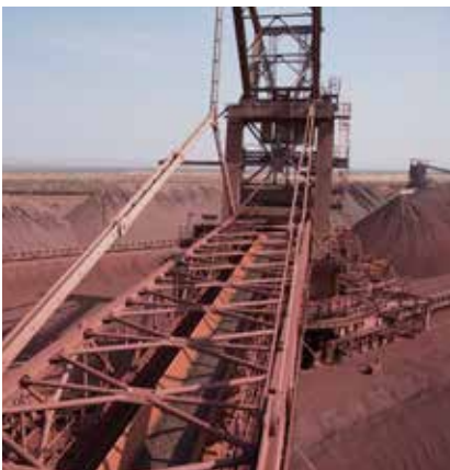
Image: Ruan Rowan, an operator doing a pre-shift inspection on Kolomela mine's reclaimer.
