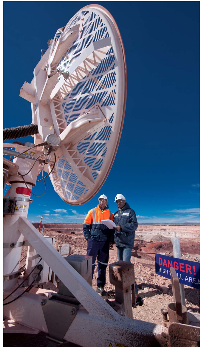
▼ Thabo Makhorele, a Technical Superintendent, and Dave Makumbila, a Senior Technician, in Geotechnical Services at the slope stability radar on the northern edge of the pit at Kolomela mine. The stability radar is mainly used to monitor any major slope changes and warns of any pit failures.
