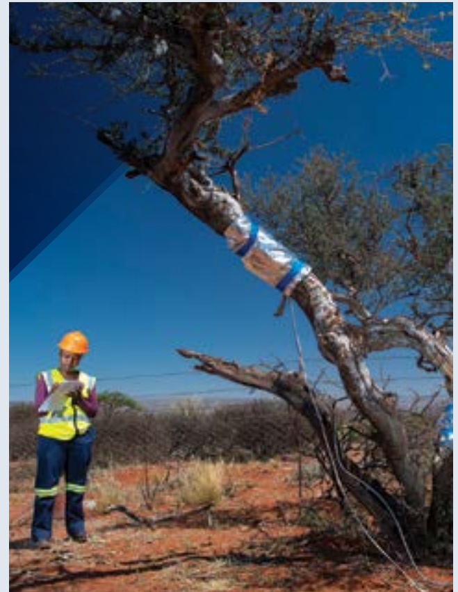
▼ Robin Bhola, an intern at Kolomela, checks on the progress of a sap flow study on the shepherd trees on the mine property. The study is conducted to better understand the tree and how it will respond if used in the rehabilitation of the mine.
