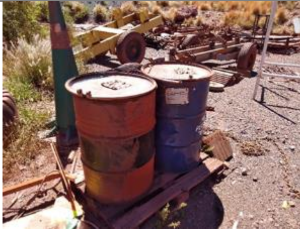
Drums not stored in demarcated & banded areas
