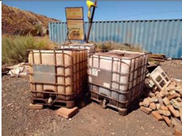
Potentially hazardous materials stored outside of a bunded area
