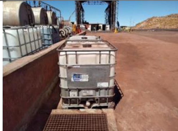
Ethylene glycol, a toxic substance, incorrectly stored outside of a bunded area
