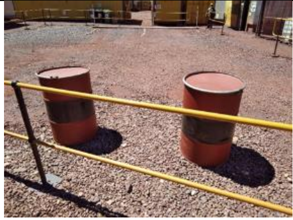
Unlabelled drums containing hazardous material.
