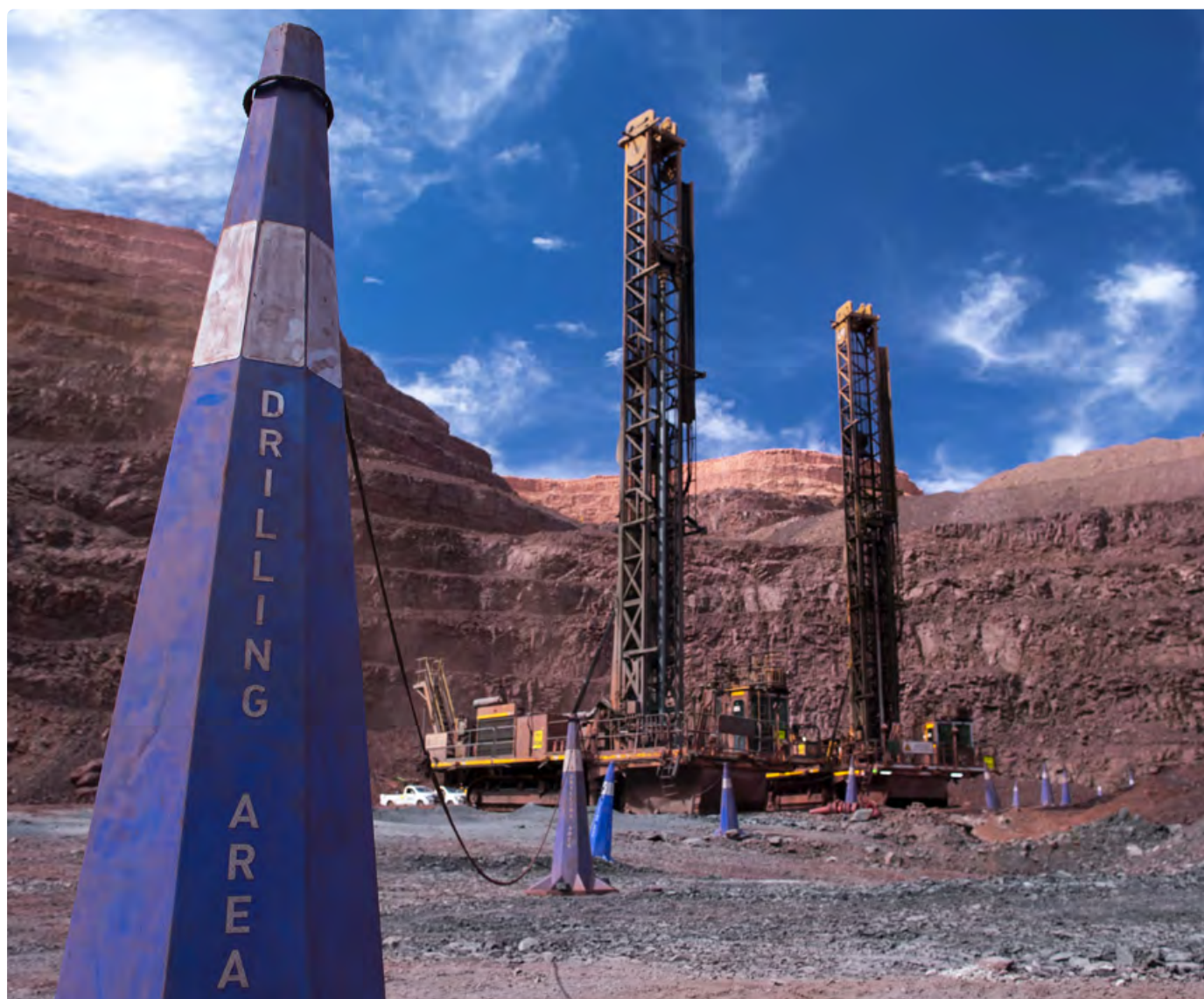
Remote operated drill rigs at Kolomela mine.
