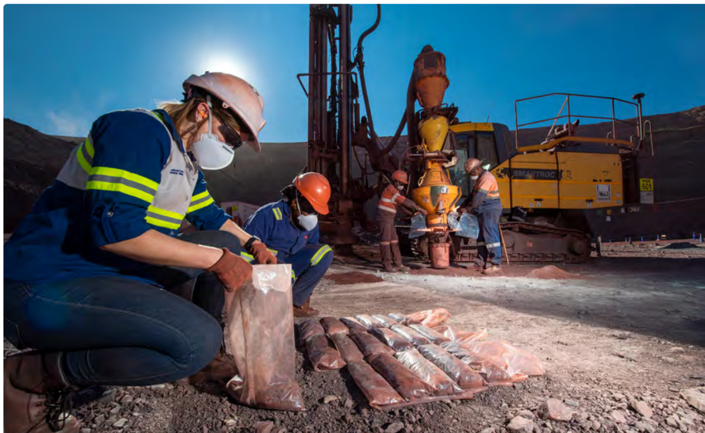
Grade control and Reverse Circulation drilling in the Leeuwfontein pit at Kolomela. Pictured here are drill operators, Bradley Mouton and Sylvester Williams, on the rig, with pit geologist Bianka Bronkhorst and sampler Manuel Legalamitlwa that will use the results from the drilling to map out the grade of the resources.
